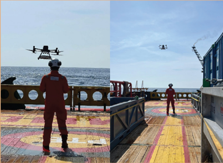
Sky-Futures Malaysia is conducting drone-based methane leak detection and measurement – Source: SFM.
