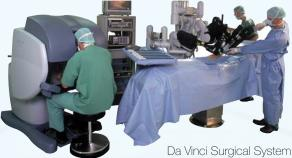
Surgical Robot : In operating theatres, robotic systems are used in both soft and hard tissue surgeries. These robots, while not yet autonomous, greatly enhance the capabilities of surgeons, allowing the surgery to be done with greater precision, using smaller incisions resulting in less blood loss and guicker healing time. They also enable remote surgeries.
