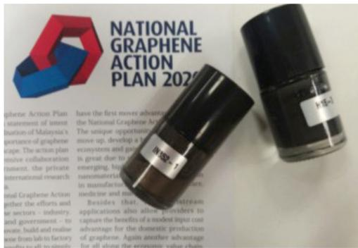
Graphene conductive ink for Radio Frequency Identification system and sensors
