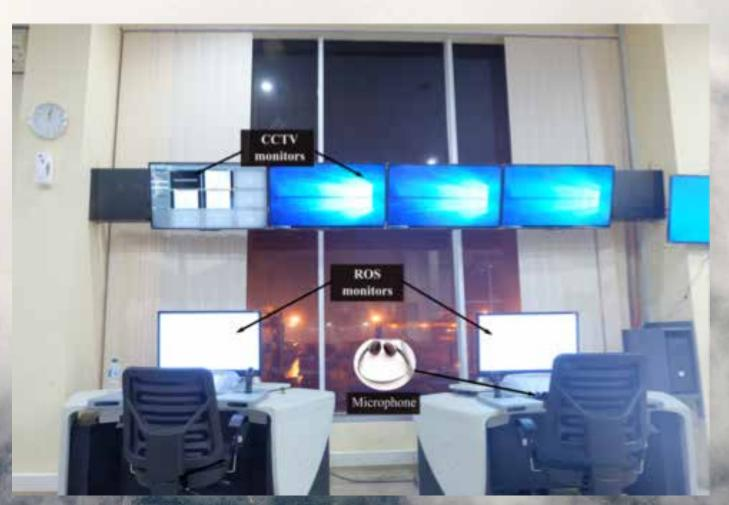
Figure 2 Remote operator station (ROS) for remote-operated crane operation
