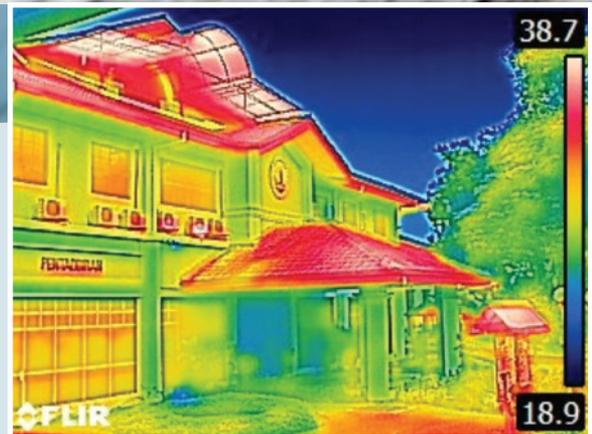
Figure 3: This thermogram shows that, generally, the roof has higher temperature compared to other parts of the building
