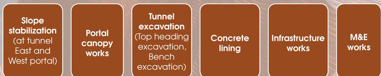
Figure 1: Stages in the construction of tunnels
