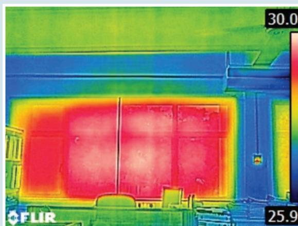
Figure 1: Glass sections of buildings have higher temperatures compared to concrete walls
